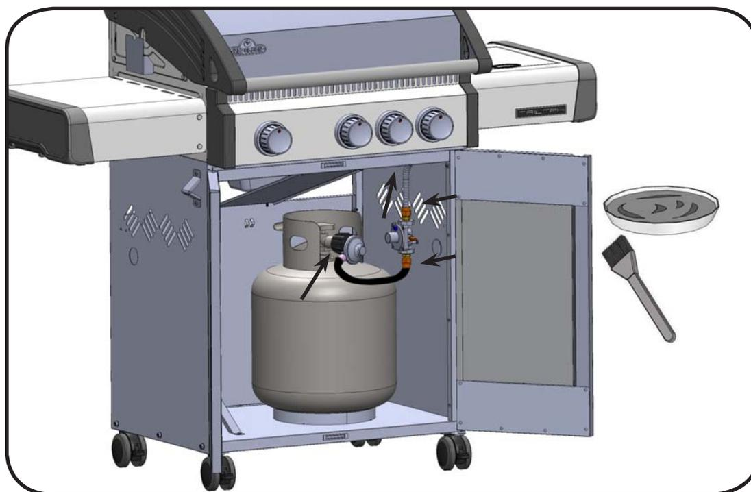
All cylinders 7kg or larger must be placed outside the enclosure (under the right side shelf) on level ground. The hose assembly must be routed through the knock out hole in the right side panel.
